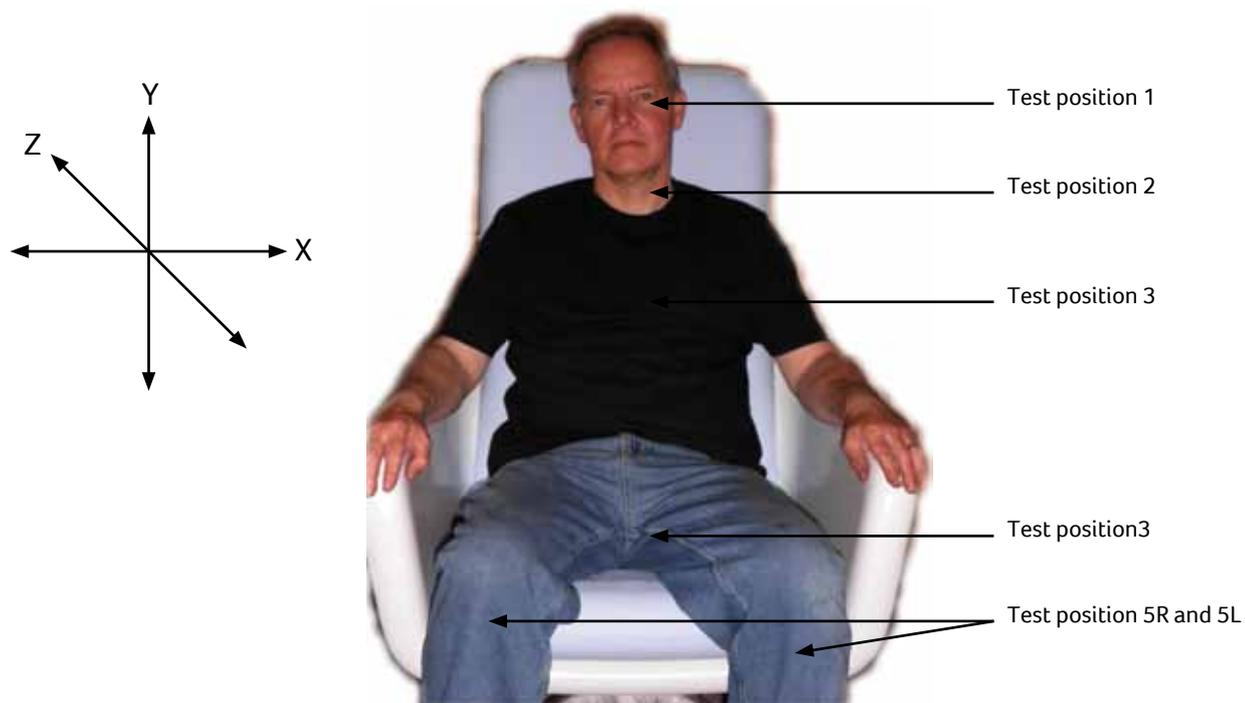
Figure 2 Person sitting in the production chair with the test positions marked
